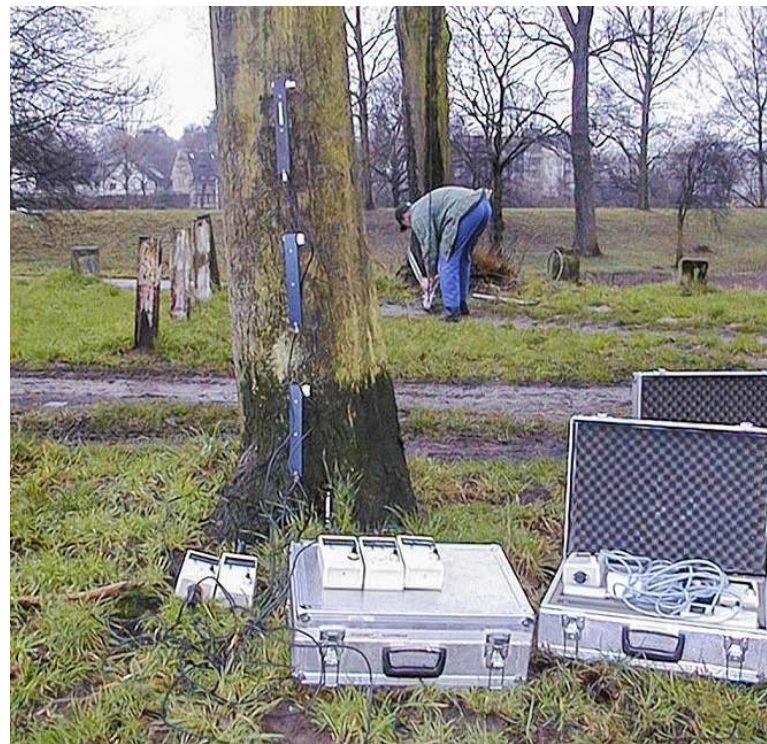
PHOTOS Stability - Inclinomethode Injury-free and safe determination of the tipping load (Wessolly 1987).
