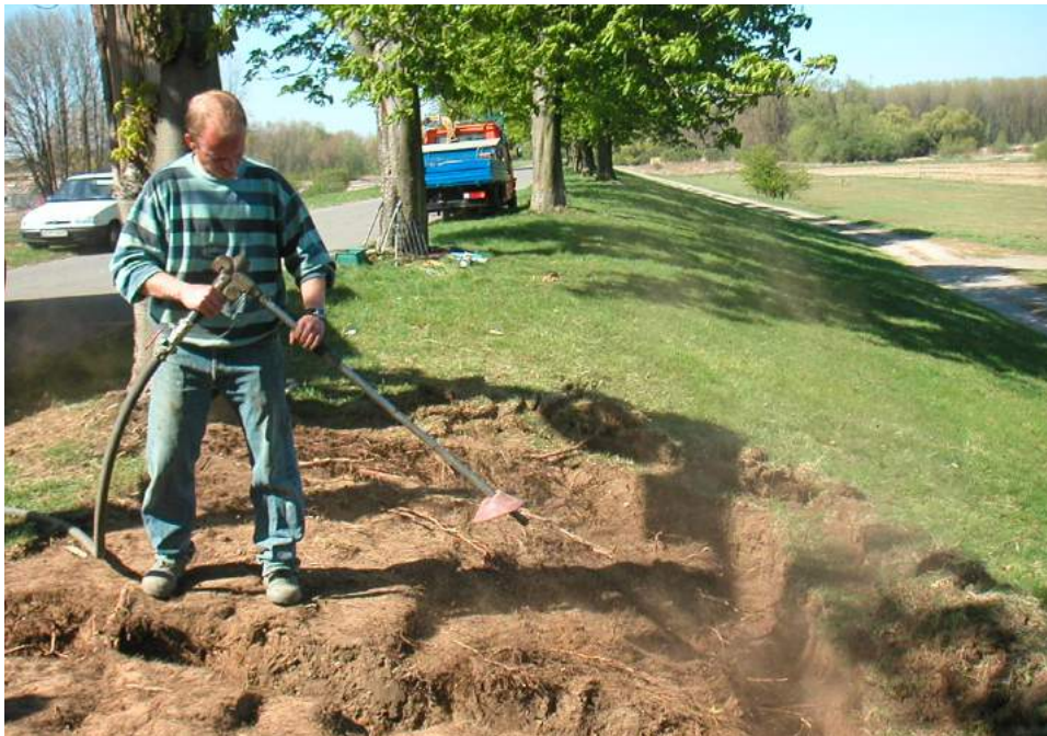
PHOTOS show the dense fine root fleece of the horse chestnut under the grass, through which not even the high-pressure flushing device could penetrate. Like a sack, this fleece holds the soil-sand mixture of the dike together, stabilizes the statics in the event of soaking and prevents rinsing (Wessolly 2002).
