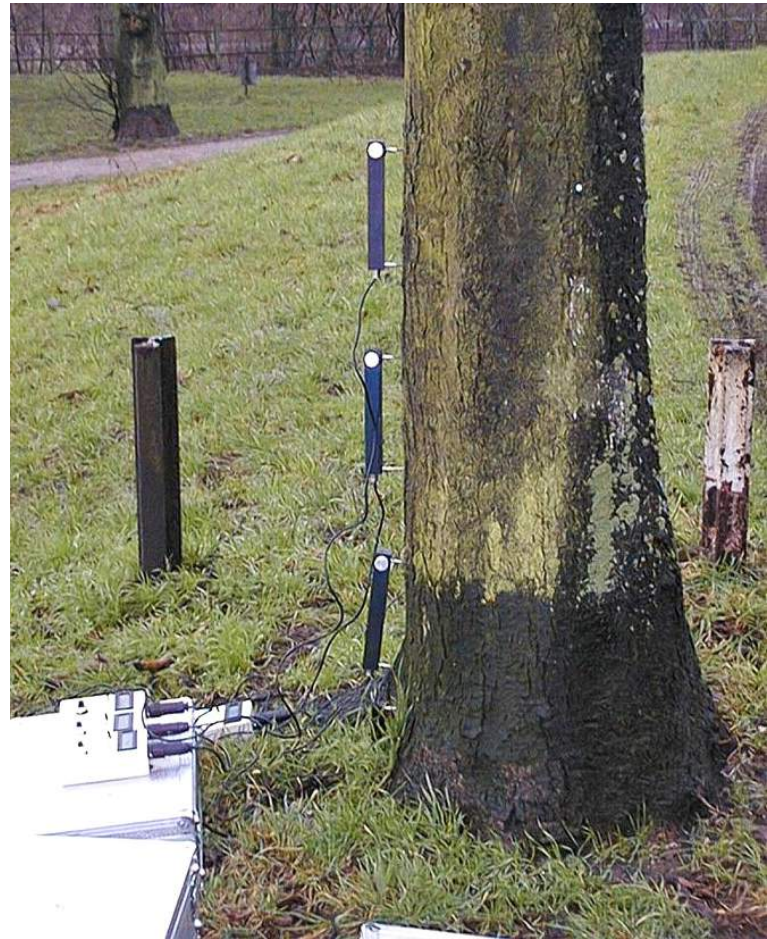
PHOTOS Stability - Inclinomethode Injury-free and safe determination of the tipping load (Wessolly 1987).
